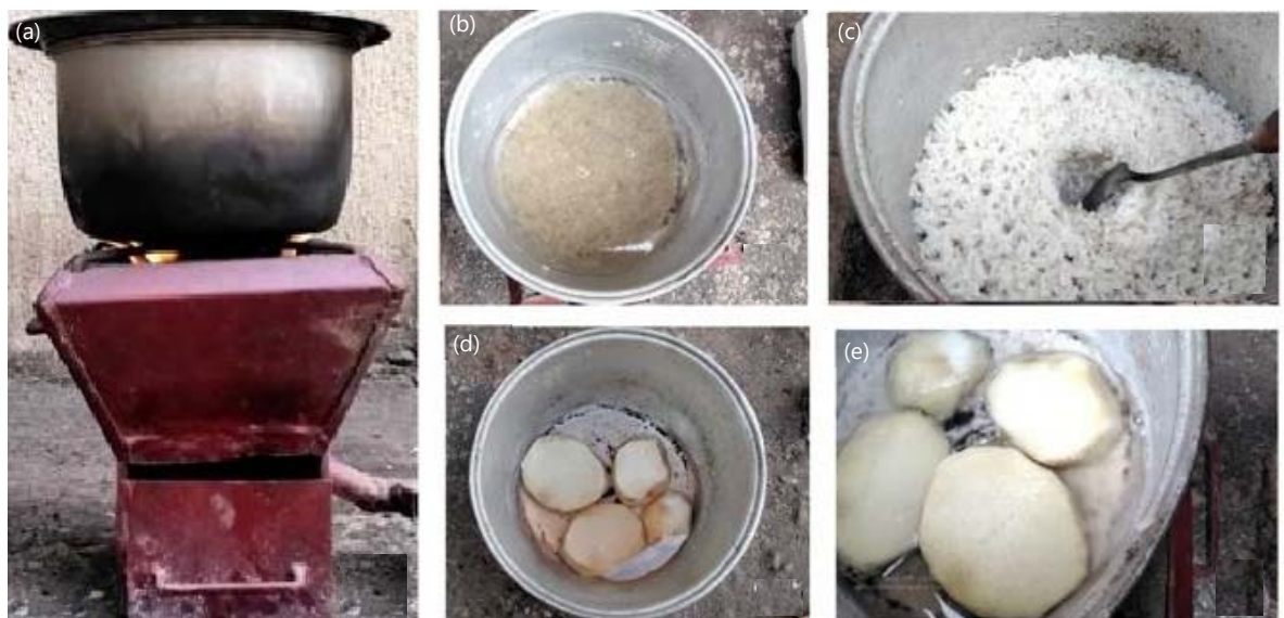
Fig. 3(a-e): WBT/CCT showing setup and products, (a) WBT/CCT setup, (b) Raw rice, (c) Cooked rice, (d) Uncooked yam and (e) Cooked yam
